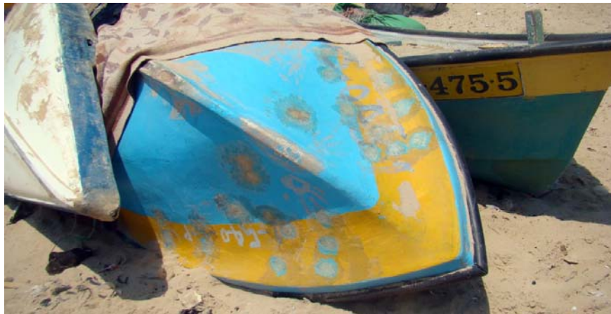
Figure 1: A fishing boat with bullet holes which have been patched with fiberglass.
